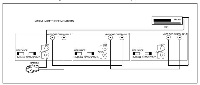
Figure 3. Monitor Looping with External Video Equipment
